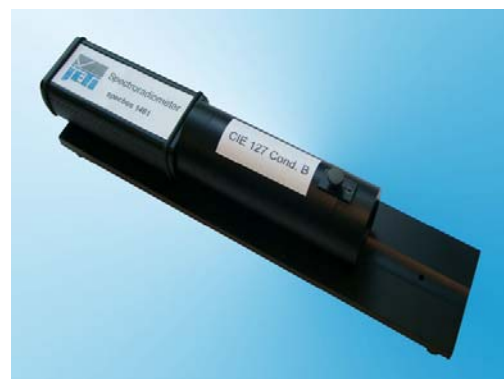
CIE condA and B tube for luminance intensity (scb1401)
