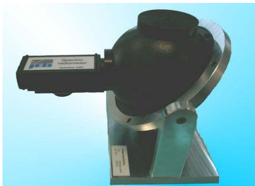
Integrating Sphere for luminance flux (scb1301)
